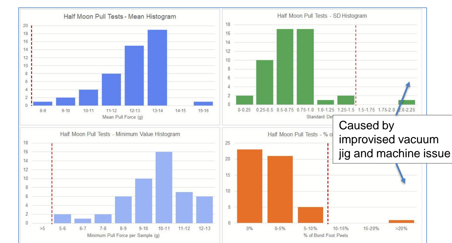
Fig: Pull test results with half moons sensor sample. 50 samples from 15 sites (barrel and endcap) [2].
