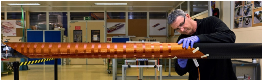
Fig. 10. Winding the first CCT prototype at CERN.
