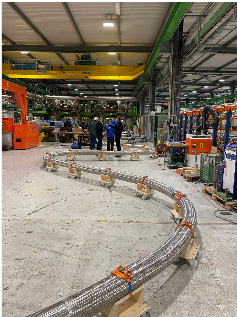
Fig. 11. Handling tests of a superconducting link.
