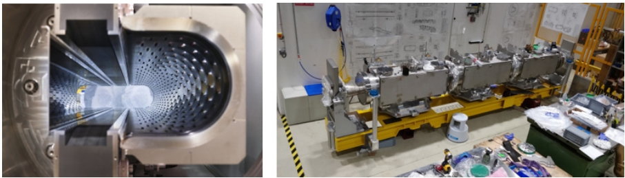
Fig. 3. Front view of the open tank of the first TDIS module (left) and side view of the three modules installed on the common girder (right).
