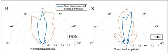
Figure 9. Directivity pattern of the acoustic source in free space (red dotted line) and in presence of the phononic crystal (blue solid line), at (a) 14 kHz and (b) 18 kHz.
