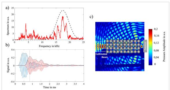
**Figure 3.** Experimental observation at 18 kHz of the endoscopic effect: (a) Spectrum of the transmitted signal for an excitation centered at 18 kHz; the dotted line denotes the Gaussian window used. (b) Transmitted time trace in solid red with the signal from the input side is shown in solid blue. (c) Snapshot of the amplitude of the integrated pressure at time t = 0.88 ms (see movie at [Multimedia 2]).
