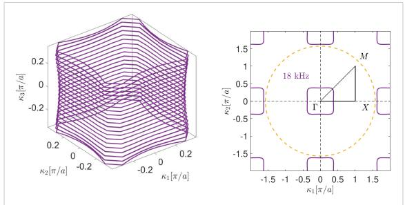
Figure 8. The isofrequency contours for the second band at 18 kHz. Left: zoomed-in 3D representation shows concentric near-squares centred around  $\Gamma$  and flat perpendicular to the  $\Gamma-X$  direction. Right: 2D representation of the isofrequency contour in the plane  $\kappa_3=0$  with the free-space isofrequency contour at 18 kHz in yellow dashed line. The large cube shown on the left panel appears as smaller squares on the right panel.
