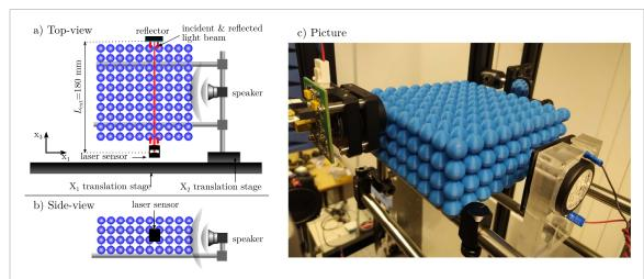
**Figure 1.** Experimental setup: the crystal and the associated acoustic source are mounted on a rigid structure built with metallic rods. The structure is moved along  $X_2$  and  $X_3$  axis using motorized translation stages while the sensor and the distant reflector remain in a fixed position. (a) Top-view. (b) Side view. (c) Photograph of the setup.
