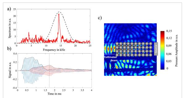
**Figure 2.** Experimental observation at 14 kHz showing endoscopic effect: (a) spectrum of the transmitted signal for an excitation centered at 14 kHz; the dotted line denotes the Gaussian window used. (b) Transmitted time trace in solid red with the signal from the input side shown in solid blue. (c) Snapshot of the amplitude of integrated pressure at time t = 1.72 ms (see movie at [Multimedia 1]).
