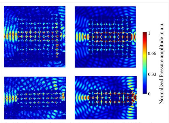
**Figure 5.** Comparison between experiments (left panels) and numerical simulations (right panels) at 18 kHz from top (upper panels) and side (lower panels) view.
