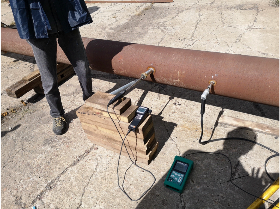
Measurement of exhaust composition. (Image: ARIES)
