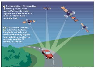
Each of the satellites has several atomic clocks that contribute very precise time data to the GPS signals. GPS receivers decode these signals, effectively synchronising each receiver with the atomic clocks, which tell time by measuring the rapid oscillations of atoms. They are so precise that they will not lose even a second of time in billions of years.
