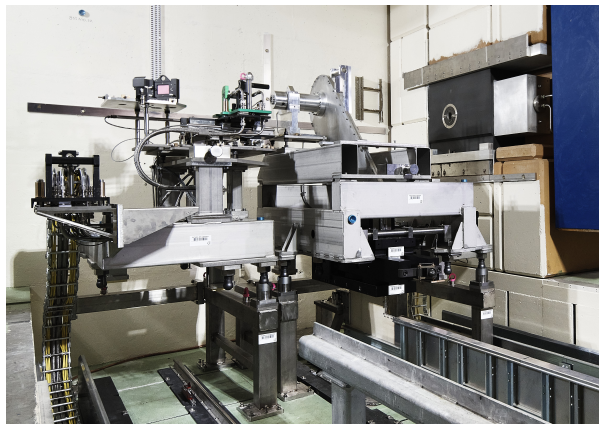
Figure 2: AD-T trolley systems of both Production target (left) and magnetic horn (right) [21].
