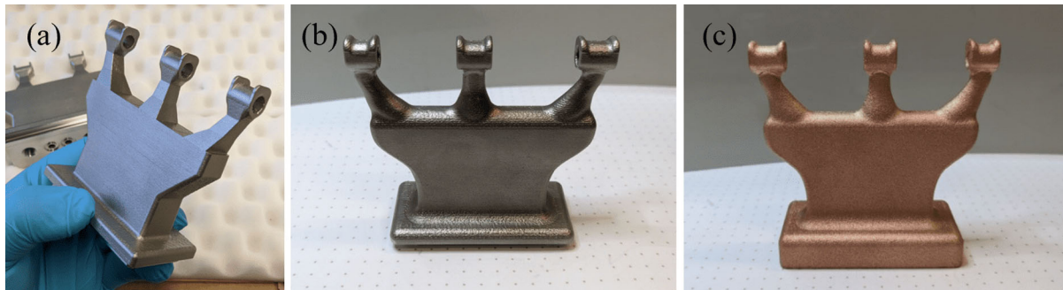
FIG. 20. Additively manufactured IH-type DTL drift tube structure made of (a),(b) 316L stainless steel and (c) pure copper [194,195].
