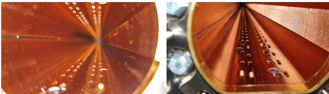
Figure 77. Photographs obtained during visual inspection of the B31L2 beam-screens (B1 left, B2 right).
