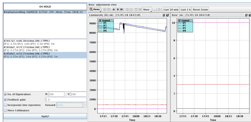
Figure 104. The operational GUI for \beta^* -levelling in “manual” mode, as used in Run 2 to reduce the \beta^* from 30 cm to 25 cm in two steps towards the end of a fill (example from fill #6714). The left part shows the available LSA beam processes and matched optics for \beta^* -levelling.
