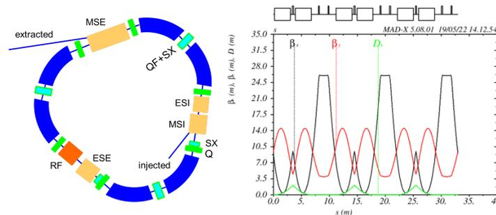
Figure 4: Sketch and optics of the He-ions synchrotron.
