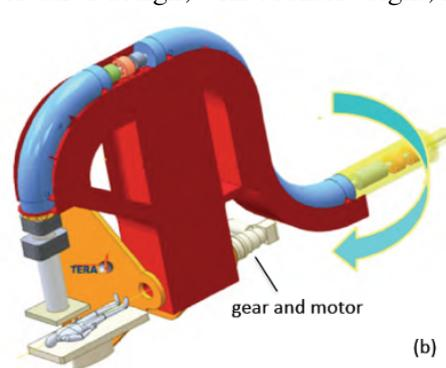
**Figure 3:** Concept of gantry attached to the wall [7]
