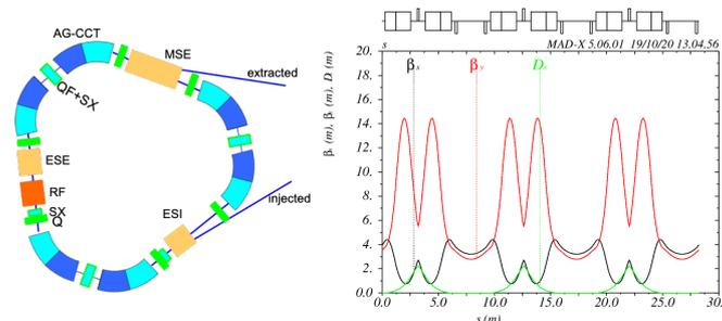
Figure 2: Sketch and optics of the SC synchrotron, triangular layout (new baseline in HITRIplus) [8]
