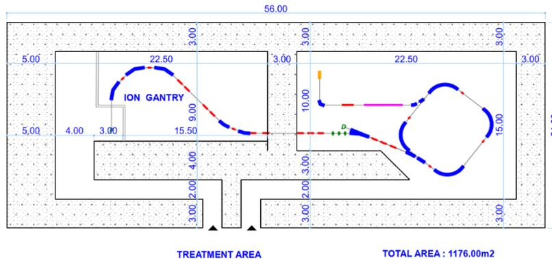
Figure 1: Layout of a compact single-room SC ion therapy facility [3].
