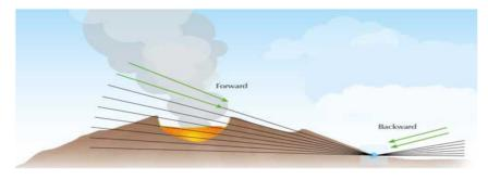
The principle of muon radiography. As they pass through the volcano, nearhorizontal muons are absorbed by the rock through which they are passing. The denser the rock, the more muons are absorbed. Backward flux is used for normalisation. Image courtesy of Nicola Graf
