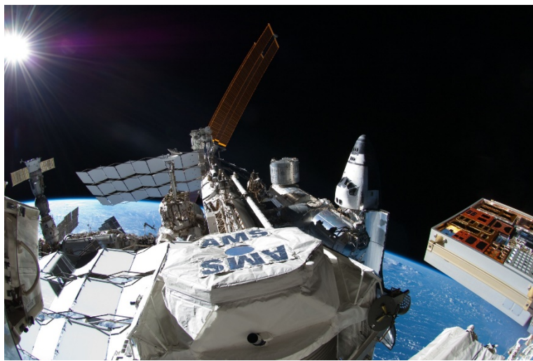
Fig. 3) AMS detector installed on the International Space Station's integrated truss structure. Image Credit: NASA
