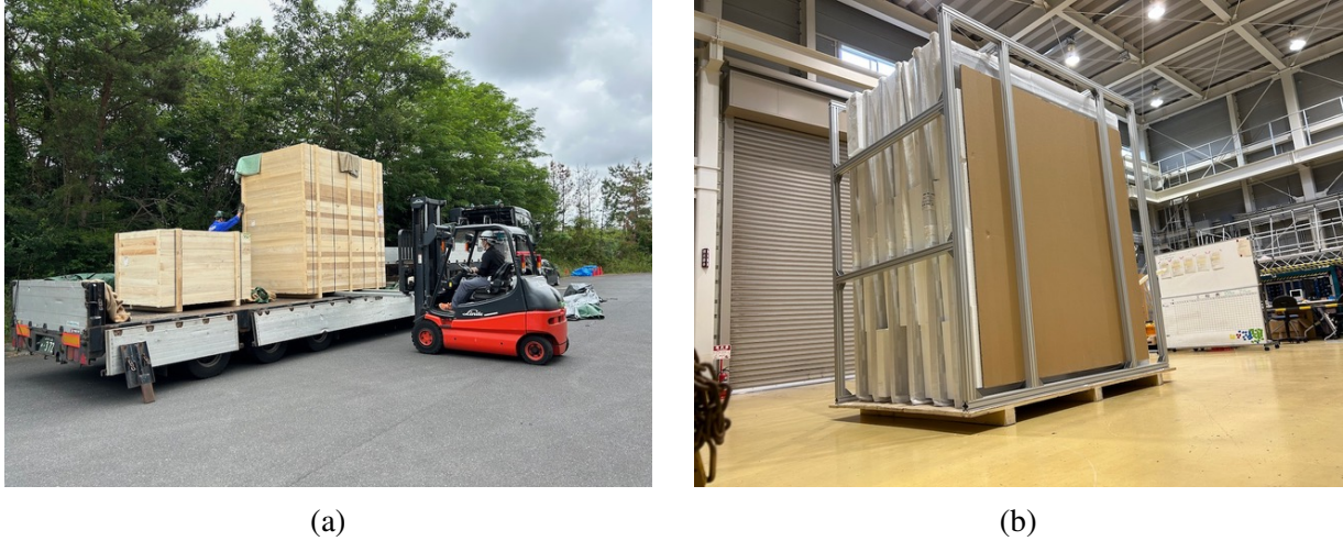
Figure 23: (a): ToF detector arriving at JPARC. (b): ToF detector just out of the box. The six modules are standing on a dedicated supporting structure.
