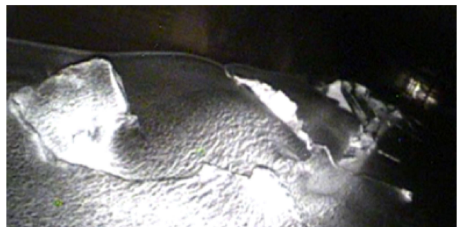
FIG. 2. Local melting of aluminum in the absorbing blocks of the TIDVG 2 beam aperture.
