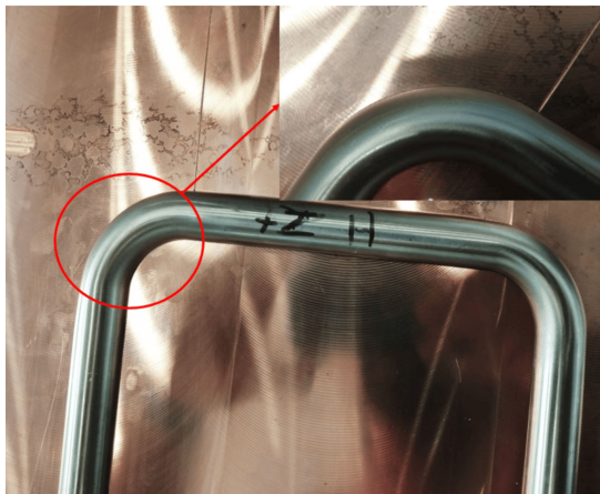
FIG. 12. Groove in CuCr1Zr plate machined with a 0.1-mm gap surrounding the tube's bend region.
