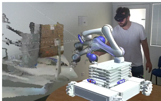
Figure 2: Operator using the CERN human-robot interface based on AR featuring a mobile platform with an attached robotic arm [26].
