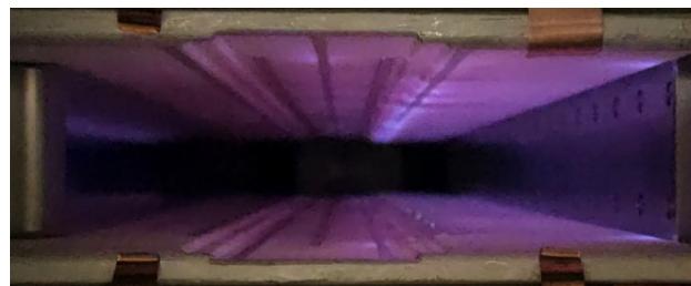
Figure 1: HV corona inside a kicker magnet.
