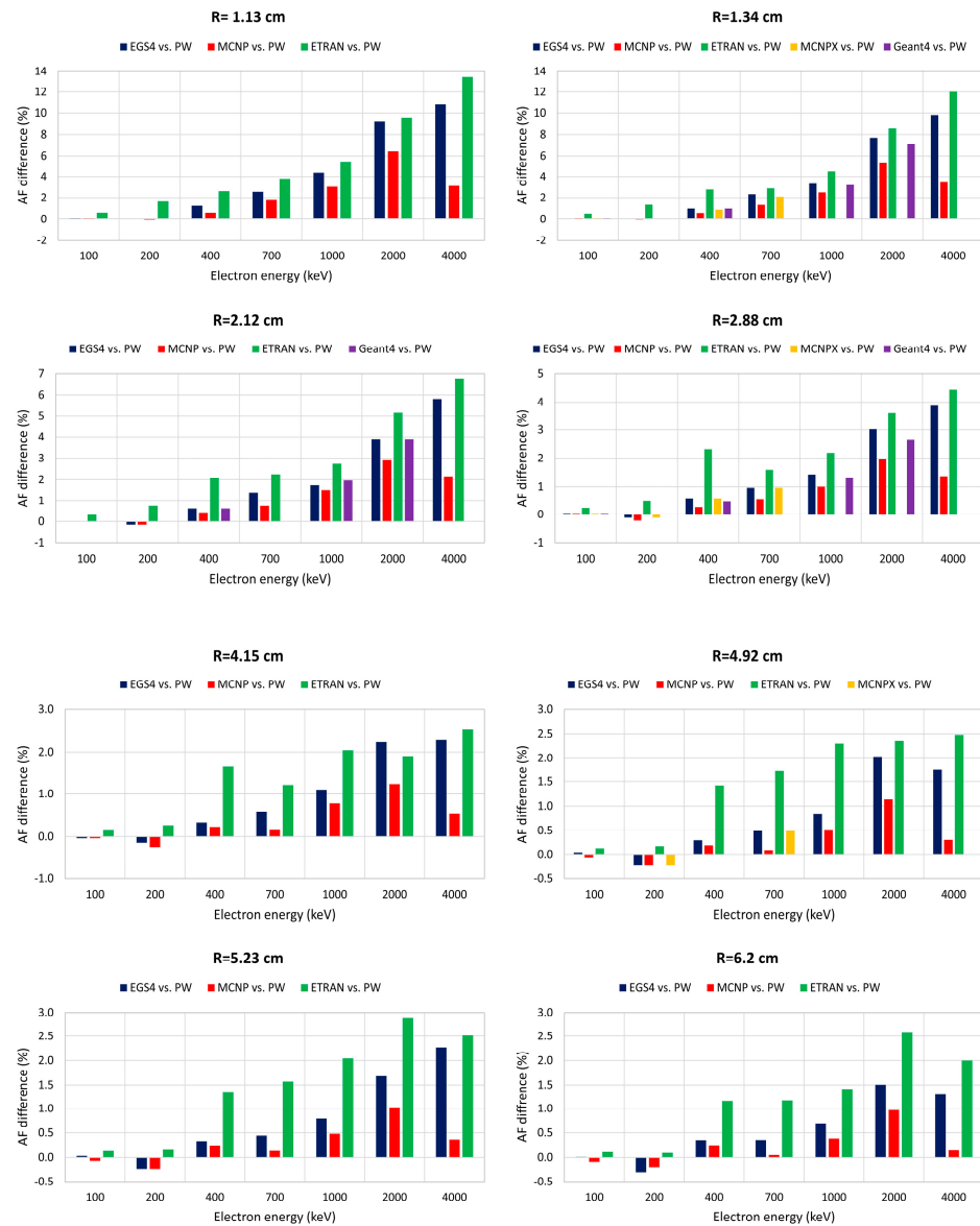
Figure 5. Percentage difference of absorbed fraction (AF) between published MC simulation data from different codes (EGS4, MCNP, ETRAN, MCNPX, Geant4) and the analytic calculations of the present work (PW), for several electron energies in the range 100 keV–4 MeV and different sphere radii (1.3 mm–6.2 cm).
