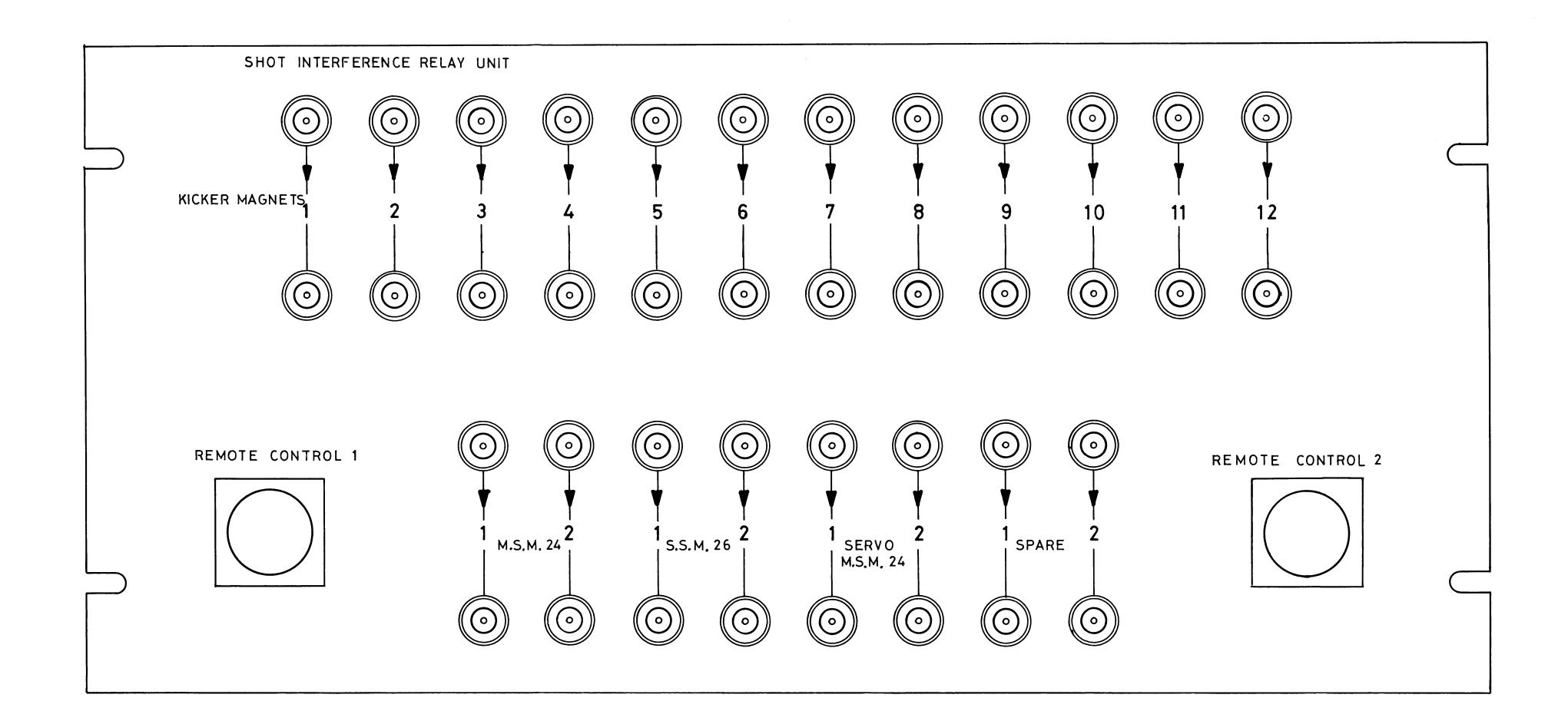
NOTE: BNC PLUGS 75Ω (ISOLATED FROM PANEL)
