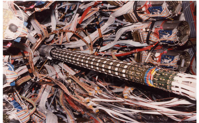
Fig. 22. UA2 inner silicon array during insertion. The little white squares are the AMPLX ASICs in their ceramic packages. (photo Claus Gößling).
