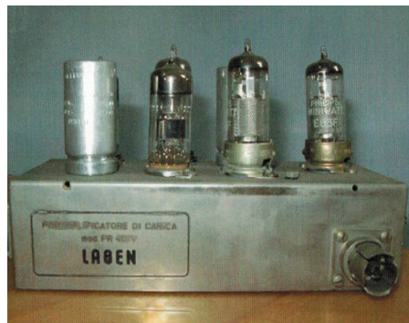
Fig. 2. Nuclear Detector Preamplifier, using vacuum tubes, ~1955. Commercialized by Laben, based on circuit designs by Emilio Gatti (photo Politecnico Milano).
