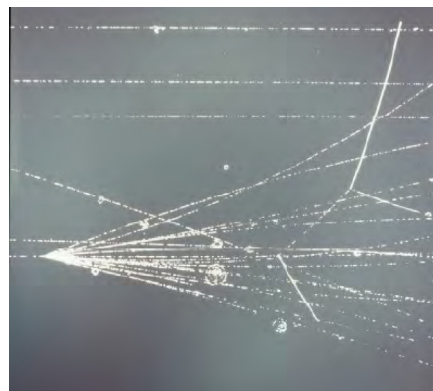
1b) beam and interaction in the 2-m CERN bubble chamber ~1970 (photo CERN)
