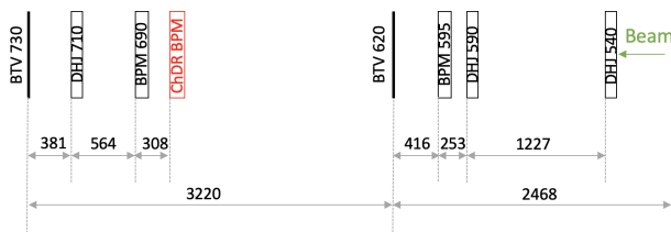
Figure 2: Schematic of the CLEAR beam-line around the location of the ChDR BPM located at \sim 7 m upstream of the end of the beam-line with distances given in mm.
