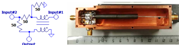
Figure 2: Resistive bridge power combiner [4]. Schematic(left) and actual device with ruler in cm (right).
