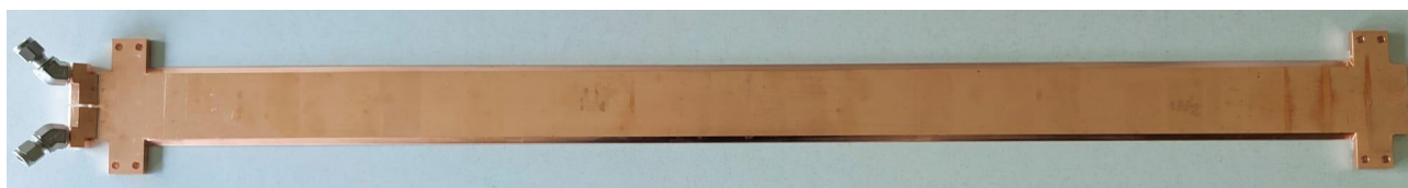
Figure 3: Photograph of the full length fourth generation septum blade (approximately 1000 mm long and weighs 2.1 kg).
