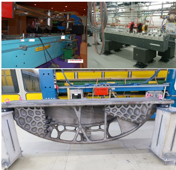
Figure 5. Top left: steel girder for SLS, courtesy M. Wurm (PSI). Top right: granite girder for SwissFEL, courtesy J. Wickstroem (PSI). Bottom: cast girder for PETRA IV [9].
