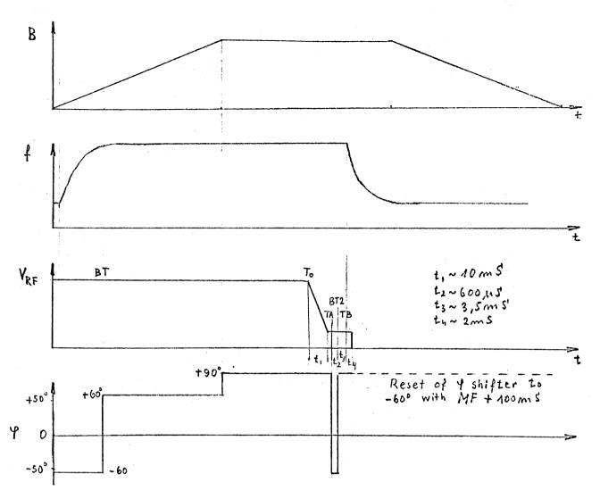
To... Start of a progressive voltage reduction (from 100% to about 20% in 10 ms),
