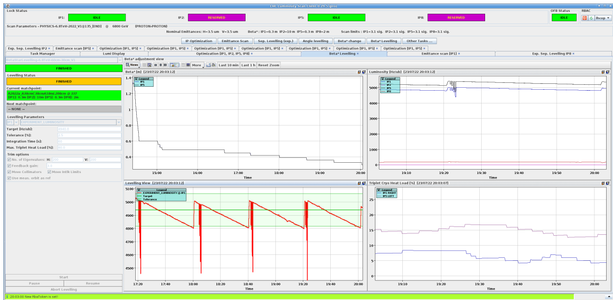
Figure 1: The operational control room application for \beta^* levelling at the LHC, after levelling from \beta^* = 60 cm to \beta^* = 30 cm in IP 1 and 5 during 2022 physics operation. The target luminosity band is shown in the bottom left panel.
