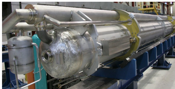
Figure 1: Q1 magnet cold mass with its overflow vessel and the bayonet heat exchanger outer shell.
