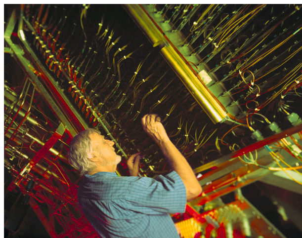
Fig. 4. Francois checking the FEE mounted on a HMPID module.
