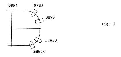
The figure 2 shows the 4 BHW dipoles for one superperiod.
