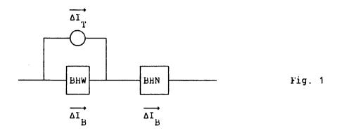
The figure 1 shows the connections of ACOl dipoles.  $\Delta I_{T}$  is the trim current variation and  $\Delta I_{B}$  is the main current variation. They are 8 BHW, 15 BHN and 1 BHS. All have the same deflection angle.
