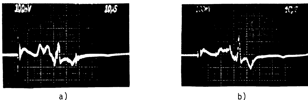
Figure 13 - Magnetic probe signals for one shot obtained simultaneously with two probes a) and b) placed at equal radius of 60 mm for 0.02 mbar argon and 4 kV charging voltage. Vertical : 100 mV/div, horizontal : 10 \mu s/div.
