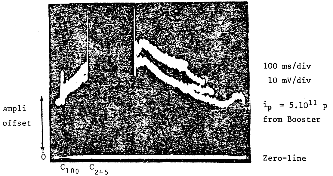
Fig. 3 Typical signal of the BCT with beam superimposed on error background.
