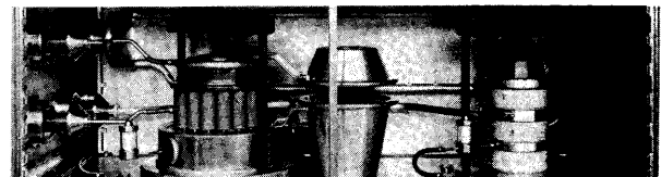
Fig. 4 Front gap (left) with pulse sharpening RC section (centre) and tail gap (right).
