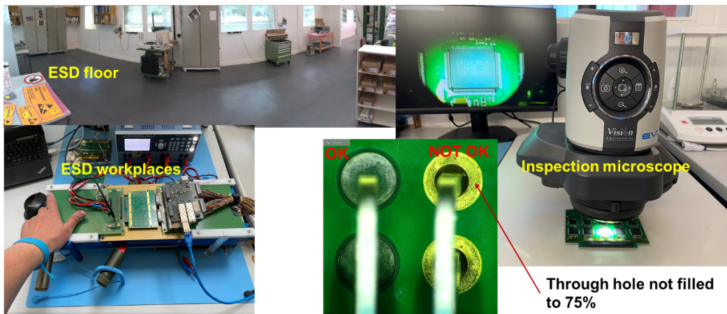
Figure 3. Images of the antistatic floor (top left) in our electronics laboratory, ESD workplace (bottom left), PCB inspection microscope (right) and insufficiently filled through hole (bottom middle).
