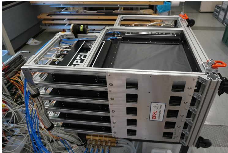
Figure 2.18: The 5 \times y SciFi tracker planes setup [61].
