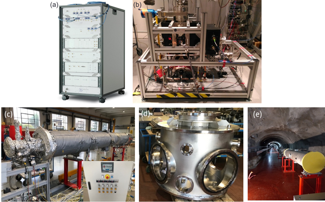
Figure 21. (a) Fibre laser system developed by the Muquans company [324], (b) cold ^{87}\text{Rb} atom source [267], (c) standard 6 m long section under vacuum test, (d) vacuum tower in production at SAES Parma (Italy), (e) MIGA gallery within the Laboratoire Souterrain à Bas Bruit (LSBB) and installation of the first sections of the vacuum vessel [325].
