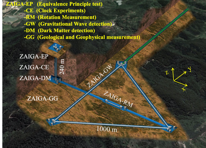
Figure 23. Layout of the ZAIGA laboratory near Wuhan, China for a range of experiments using atom interferometry [7].
