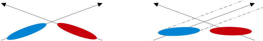
Fig. 2. Bunches colliding with a crossing angle without crab crossing (left); with the crab crossing (right).
