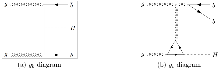
Figure 1: Sample Feynman diagrams for b\bar{b}H production proportional to y_b at tree-level and proportional to y_t induced by a top-quark loop.
