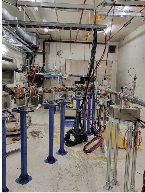
FIG. 35: Photo of Fermilab MeV Test Area showing 400 MeV proton beamline at right and pion–muon quadrupole channel at left. The protons enter traveling into the page at the right edge of the photo, and muons (produced both within the target and via pion decay in flight) exit out of the page at the left edge. A target holder is situated at the intersection of the two beam lines, followed by a small solenoid to capture charged particles produced in the target.
