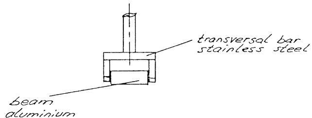
The difference in elongation between the transversal bar in stainless steel and the aluminium beam during cool-down is taken up by a spring. This causes a reaction force on the leaf-spring. This force is calculated to be 160 N. The stress in the leaf-spring is then:
