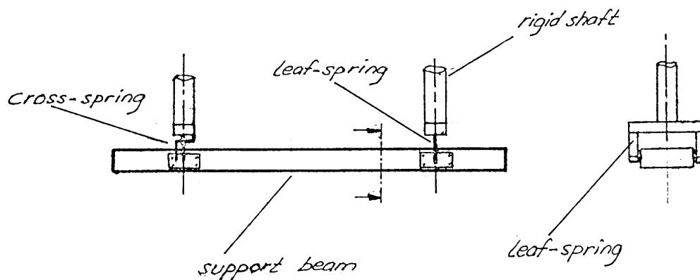
Figure 1: The electrode support beam
