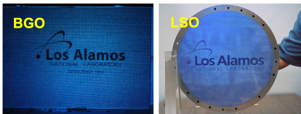
Fig. 10: Segmented BGO and LYSO [94] scintillators. Both have 1\text{ mm} \times 1\text{ mm} \times 40\text{ mm} scintillator pixels and are separated by a metal septum.
