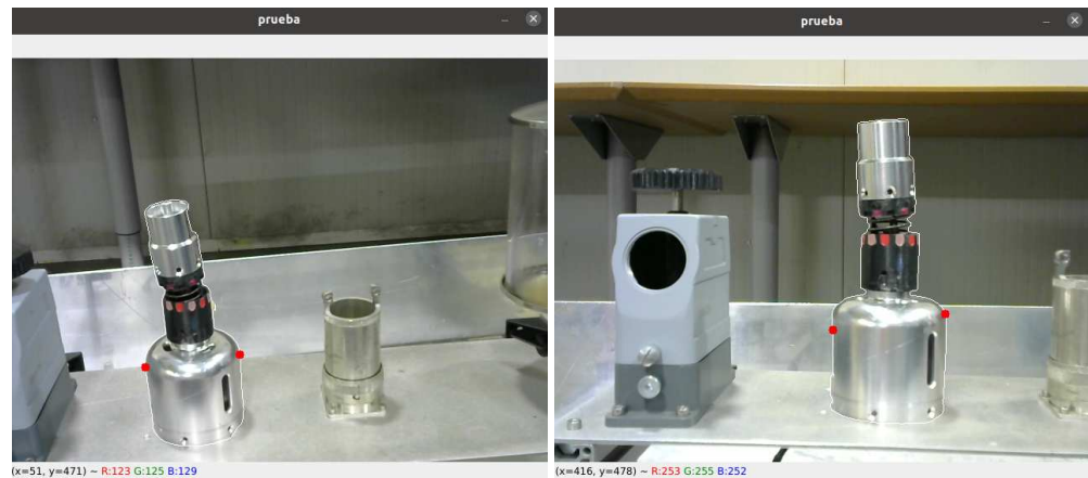
Figure 20. Determination of the grasping points of an element from various perspectives to assess the repeatability of the algorithm.
