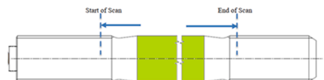
Fig 2. Schematic of the configuration of the UT inspection by immersion. The controlled region is depicted in green.
