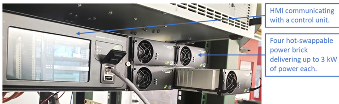
Figure 2. Device under test purchased from Eltek consisting of main functional blocks of a large-scale system providing up to 1 MW of power.
