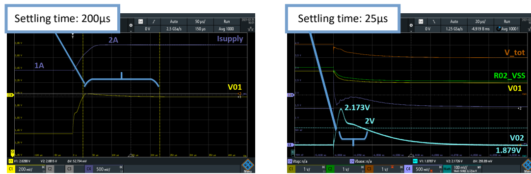
Figure 7. Single Regulator: settling time limited by large RC time (left). Serial chain: OVP limits overvoltage (right).
