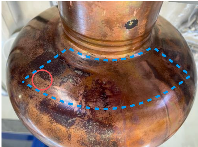
FIG. 19. Picture of the outer surface of the Nb/Cu cavity in correspondence with the cold area, which is observed during the cavity tests at 2.4 K at saturation pressure.
