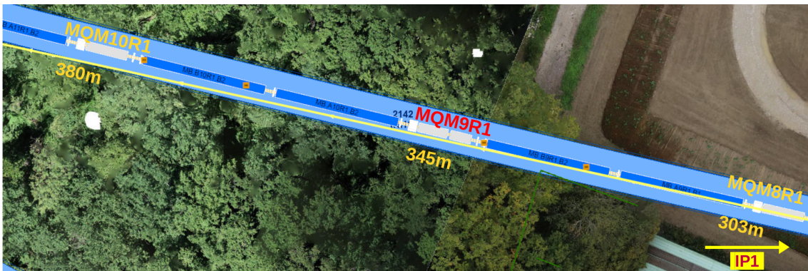
Figure 30: Map of the LHC area where Beam 1, the clock-wise circulating beam moving from right to left in this figure, is bent in the LHC arc at half-cell 9. The light yellow line shows the ATLAS detector axis. Abbreviations denote the quadrupole magnets of the corresponding half-cells. The marked distances are with respect to IP1. The latter lies further on the left, outside of the map. The original image is from the CERN GIS portal [24].
