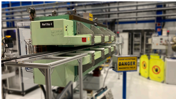
Fig. 9. Normal conducting dipole magnet and the moving fluxmeter installed for midplane measurements.
