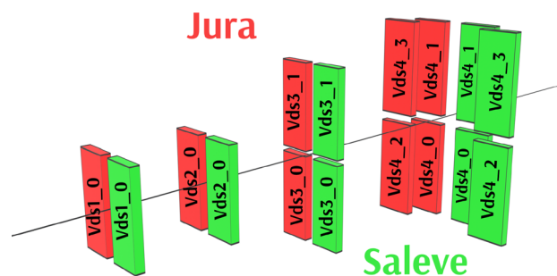
Fig. 4 The naming convention of the SAVD sensors. The first number following “Vds” denotes the station, while the second gives the sensor number in a given station
