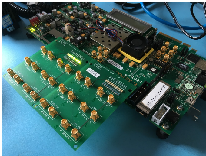
Fig. 5. SMA to FMC converter cards interface with TLU Kintex-7.
