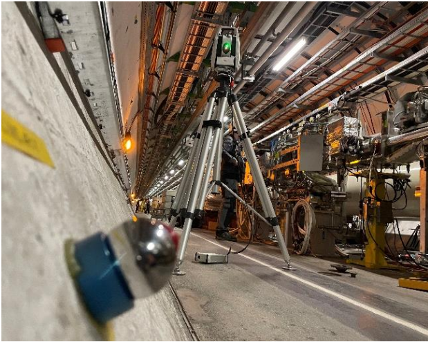
Figure 3: Laser tracker measurement on a CERN nest
