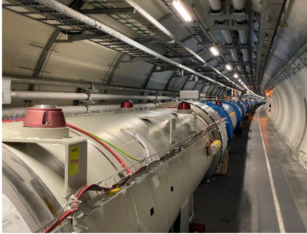
Figure 2: LHC Arc view with cryo-dipole in bleu and cryo-quadrupoles in white
