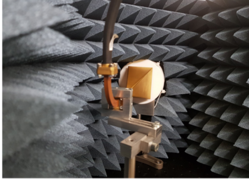
Figure 3.37: Initial part of the signal acquisition system for the ChDR theory verification experiment.
