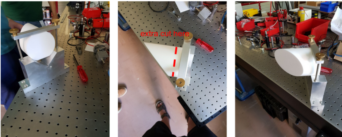
Figure 3.34: PTFE Radiator used for experimental verification of ChDR models.
